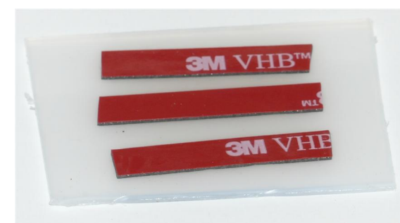
Tape to secure wires.
